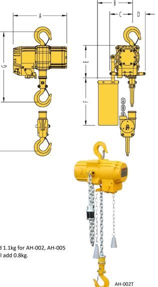
\* Weight of TAHS model includes 3m lift, 2m toggle control. For longer lifts add 1.1kg for AH-002, AH-005 and AH-010 models and 2.2kg for AH-020 per metre of lift. For pendent control add 0.8kg.
