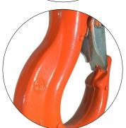
Our drop forged and heat treated alloy hooks are furnished with heavy duty spring latch kits that fully engage into the recessed nose of the hook safeguarding the load when side loading of the latch occurs and offering maximum load security. The swivel hooks are attached to the yoke using high grade nuts & bolts allowing for complete inspection during any statutory inspection or written scheme maintenance.
