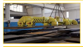
Lifting beams (with or without telescopic arms) able to handle sheets of different sizes, and of small (2mm) or greater thicknesses.
