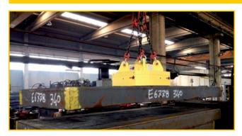
The well-structured SEP lifters, specially designed for the handling of slabs and forged blocks with an increased air-gap, are able to withstand high stresses and strains and are therefore extremely reliable over time.
