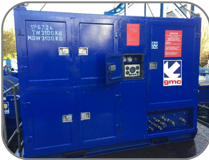
80 kW zone 2 electric HPU
