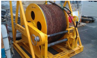
5 Ton manual winch 50 T holding
