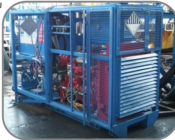
63 kW safe area diesel HPU
