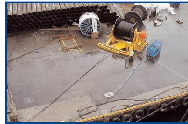
Change of anchor wire for «Safe Caledonia», drum 60T, 15T back tension
