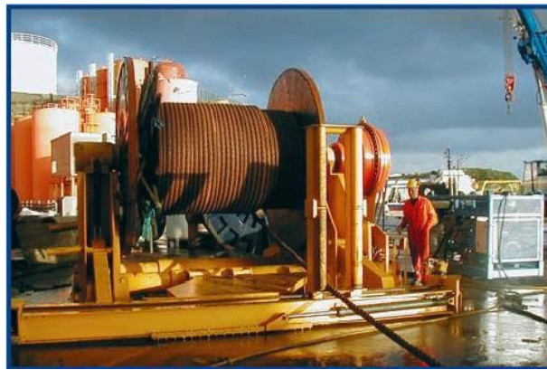
Change of anchor wire for «Safe Caledonia», drum 60T, 15T back tension
