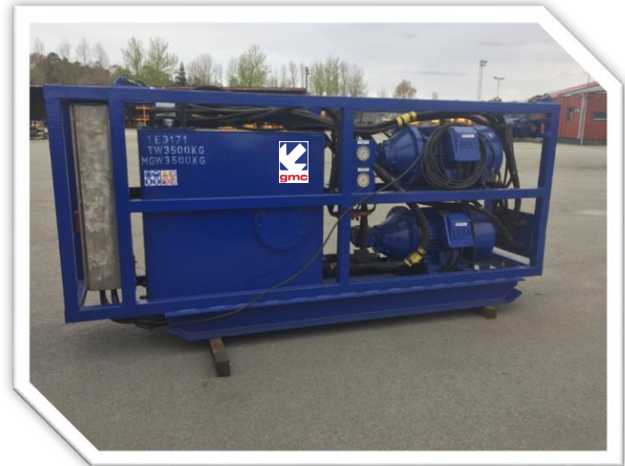
2 x 55 kW twin safe area electric HPU
